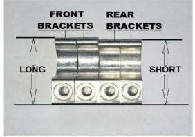
Install one of the rear brackets loosely on the skid plate and then hook the bracket in its position over the frame rail. Place the remaining rear bracket into position on the frame rail / skid plate and thread both mount bolts in finger tight for now. Place each front bracket into position and thread both mount bolts in finger tight for now. Confirm the skid plate is properly positioned and press the skid plate up against the frame rails while tightening all four bolts to 9-12 ft/lbs.
